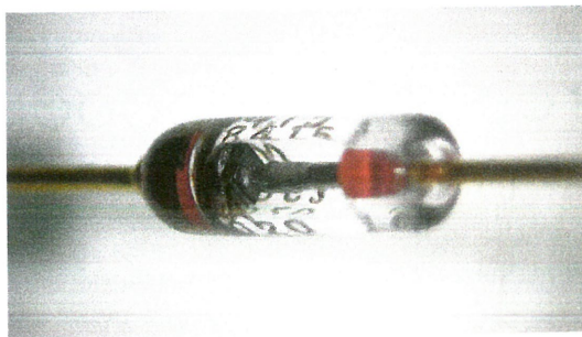
Figure 1-8. A silicon diode, the square silicon crystal can be seen between the two leads.
